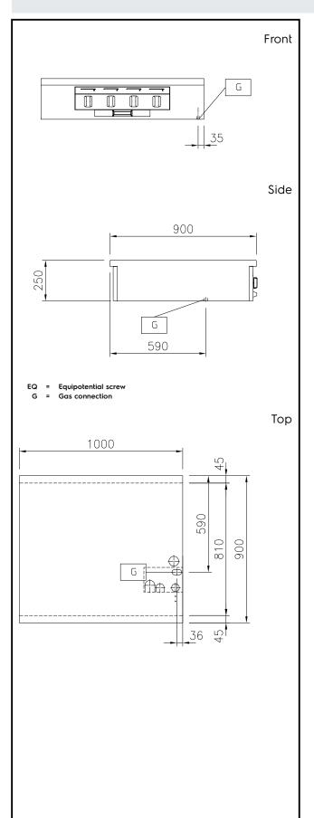
Gas Gas Power: 34 kW Gas Type Option: Gas Inlet: 1/2" **Key Information:** External dimensions, Width: 1000 mm External dimensions, Depth: 900 mm External dimensions, Height: 250 mm Net weight: 82 kg Configuration: One-Side Operated;Top Front Burners Power: 8.5 - 8.5 kW **Back Burners Power:** 8.5 - 8.5 kW **Back Burners Dimension -**Ø 70 Ø 70 mm Front Burners Dimension -
